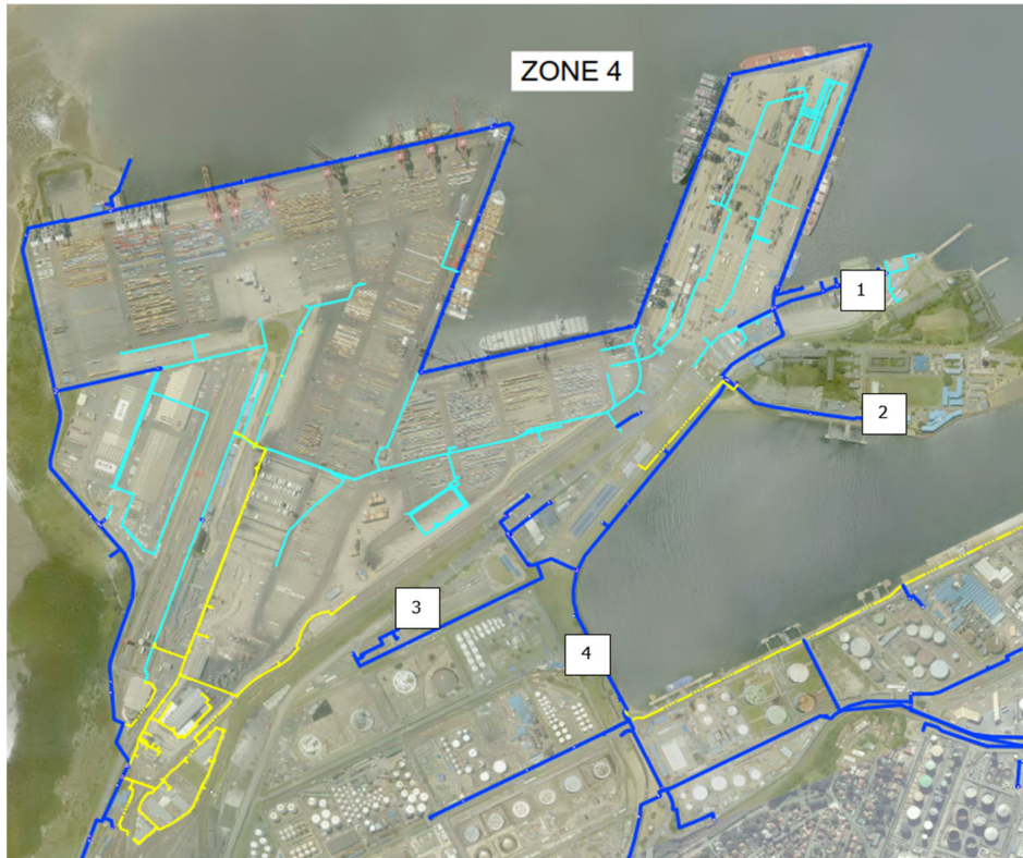
Zone 4 pipe work shown with possible positions of pressure transmitters.
