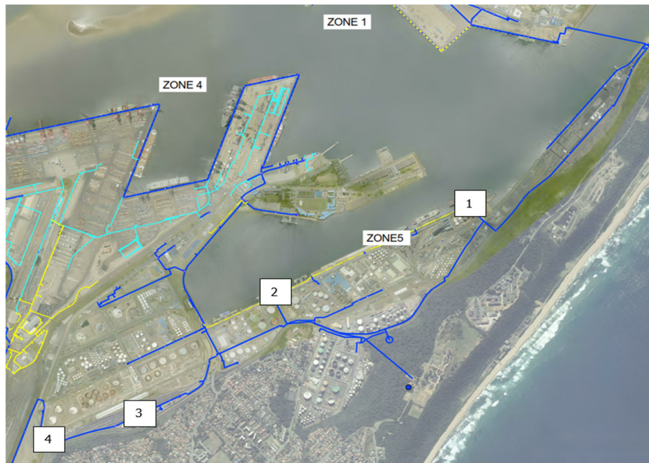
Zone 5 pipe work shown with possible positions of pressure transmitters.
