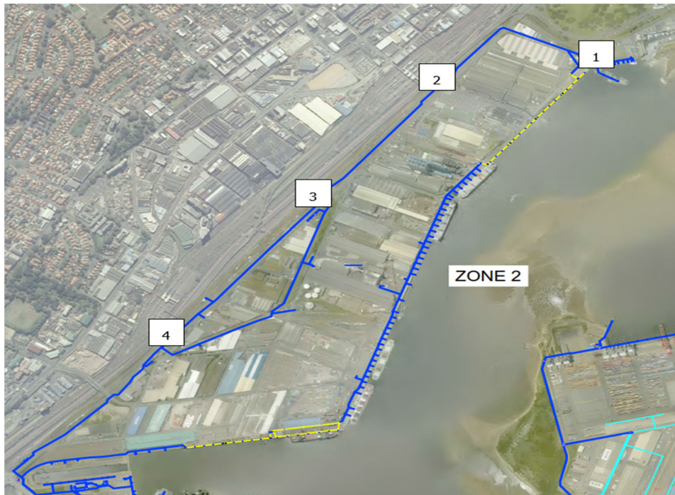
Zone 2 pipe work shown with possible positions of pressure transmitters.
