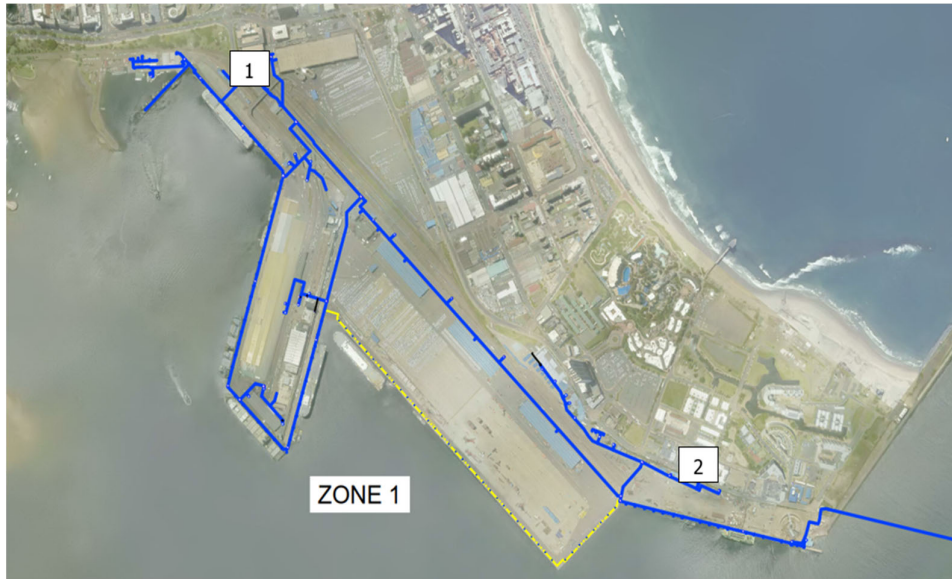
Zone 1 pipe work shown with possible positions of pressure transmitters.
